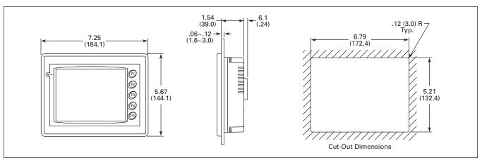
Figure 9. HMI06\_\_ — Approximate Dimensions in Inches (mm)
